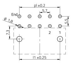
Recommended PCB layout thickness : 1.6 mm
