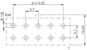
Recommended PCB Layout Thickness: 1.6mm General Tolerance ± 0.05 mm
