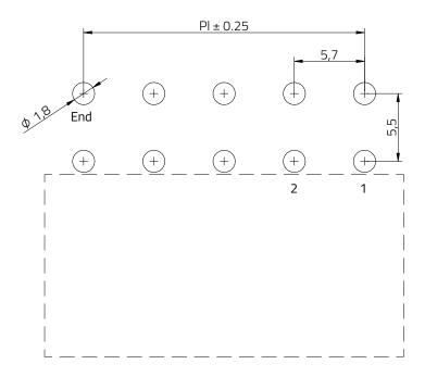
Recommended PCB Layout Thickness: 1.6 mm General Tolerance: ± 0.05 mm
