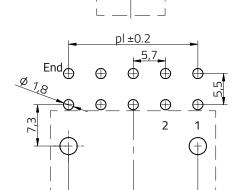
Recommended PCB layout thickness : 1.6 mm
