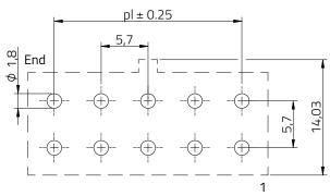
Recommended PCB Layout Thickness: 1.6mm General Tolerance ± 0.05 mm
