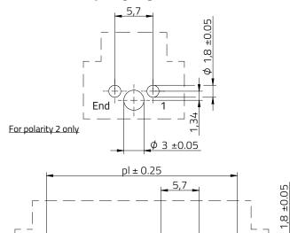
Recommended PCB Layout Thickness : 1.6 mm General tolerance ± 0.05 mm
