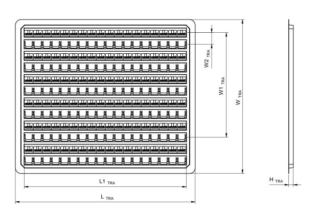
Cover Α - Tray detail A Row cavity Embossment CHECKED REVISION DATE (YYYY-MM-DD) GENERAL TOLERANCE PROJECTION METHOD MPI 002.000 2022-08-30 DIN ISO 2768-1m DESCRIPTION **WR-BHD Female IDC Connector** ORDER CODE 62504423021 SIZE/TYPE BUSINESS UNIT STATUS PAGE
