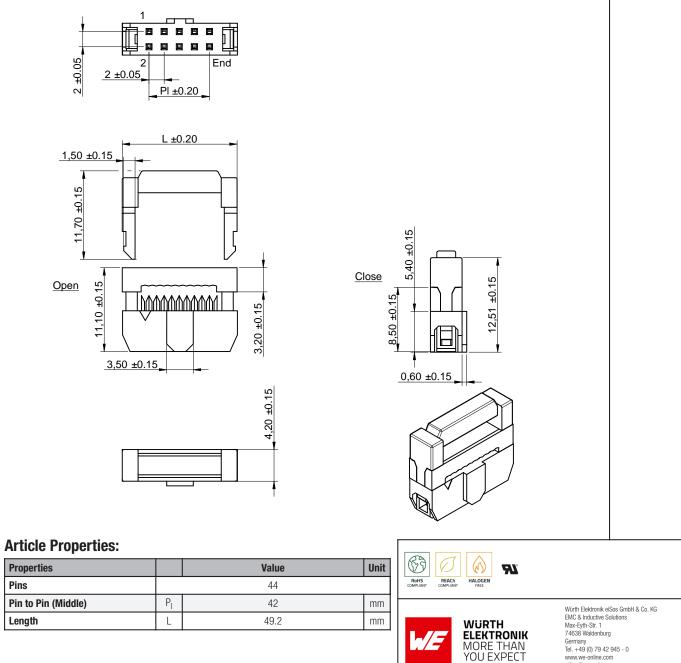
CHECKED DATE (YYYY-MM-DD) GENERAL TOLERANCE PROJECTION METHOD REVISION  $\oplus$ MPI 002.000 2022-08-30 DIN ISO 2768-1m DESCRIPTION **WR-BHD Female IDC Connector** ORDER CODE 62504423021 SIZE/TYPE STATUS BUSINESS UNIT PAGE with Strain Relief, 2.00 mm eiCan Valid 1/6
