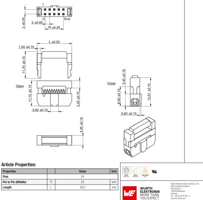
CHECKED DATE (YYYY-MM-DD) GENERAL TOLERANCE PROJECTION METHOD REVISION Ð MPI 002.000 2022-08-30 DIN ISO 2768-1m DESCRIPTION **WR-BHD Female IDC Connector** ORDER CODE 62502423021 SIZE/TYPE STATUS BUSINESS UNIT PAGE with Strain Relief, 2.00 mm eiCan Valid 1/6
