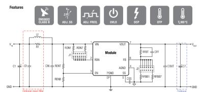
The additional aluminium electrolytic capacitor C1 is only for evaluation board protection purposes. It is mounted at the termination of the supply line and provides slight damping of possible oscillations of the series resonance circuit represented by the inductance of the supply line and the input capacitance. It is not essential for operation. The switching frequency of the module can be additsted by changing the position of immer J1.
