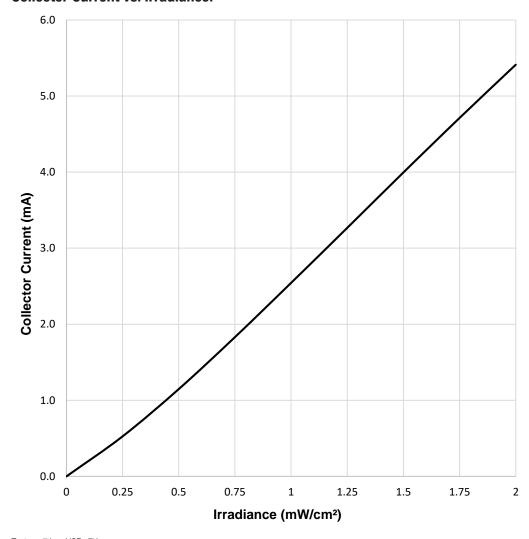
Testcondition: Ee=0,5mW/cm<sup>2</sup>, VCE=5V
