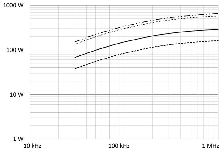
All curves are DC-DC unless otherwise noted. For offline applications, the power level must be derated as shown in the flyback curves.
