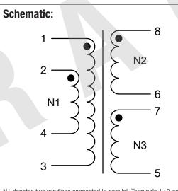
N1 denotes two windings connected in parallel. Terminals 1+2 and 3+4 must be tied as solder bridging is allowed.
